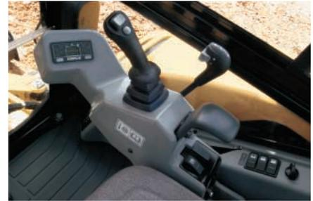
**Low Effort Controls.** Ergonomic, low effort controls offer greater operator comfort for increased productivity. Dozer lever mounted, two-speed travel control provides easy operation and increases foot room.
